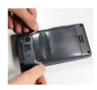
2. Grab the battery cover by the sides and lift it out of the way:
